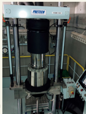
High-pressure hydrogen gas atmosphere machine for material testing (Installed at HyTReC)
