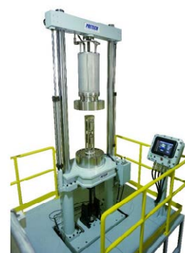
Hydrogen embrittlement evaluation equipment scheduled for installation (example)
