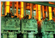
Began operation of vertical, round cross section continuous caster (No. 2 CC) in 1992
