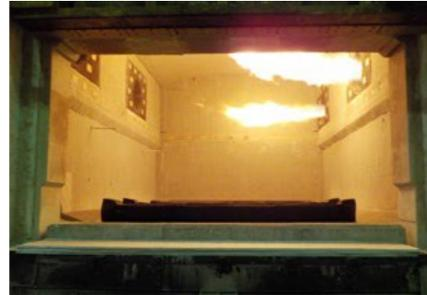
Application of a low-emissivity heat resistant paint to heating furnaces
