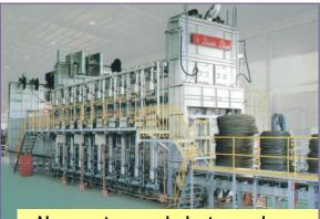
Non-water-cooled atmosphere heat treatment furnace
