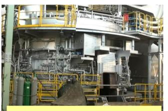
STARQ (Arc furnace with a rotation drive)
