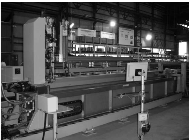
Fig.5. Appearance of high precision ultrasonic inspection system for steel bars.
