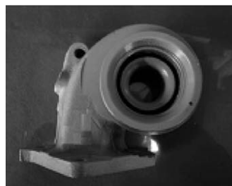
Fig.18. Appearance of turbine housing.
