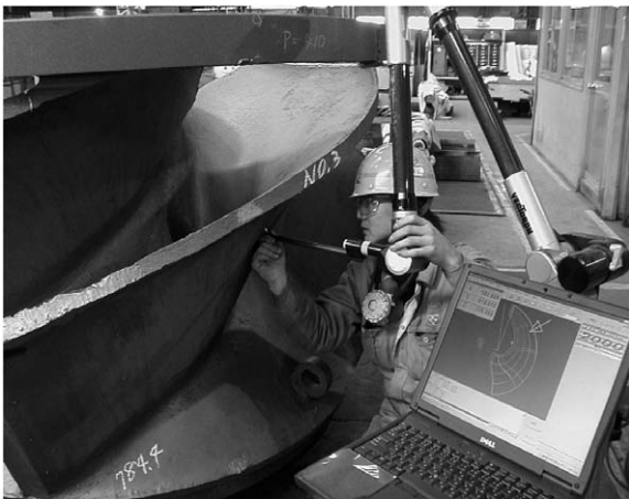
Fig.6. Measurement of three-dimensional shape of an impeller with six joints spatial coordinate meter.
