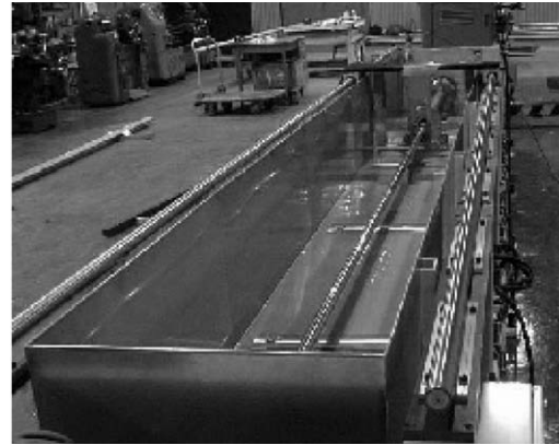
Fig.12. Appearance of immersion tank.
